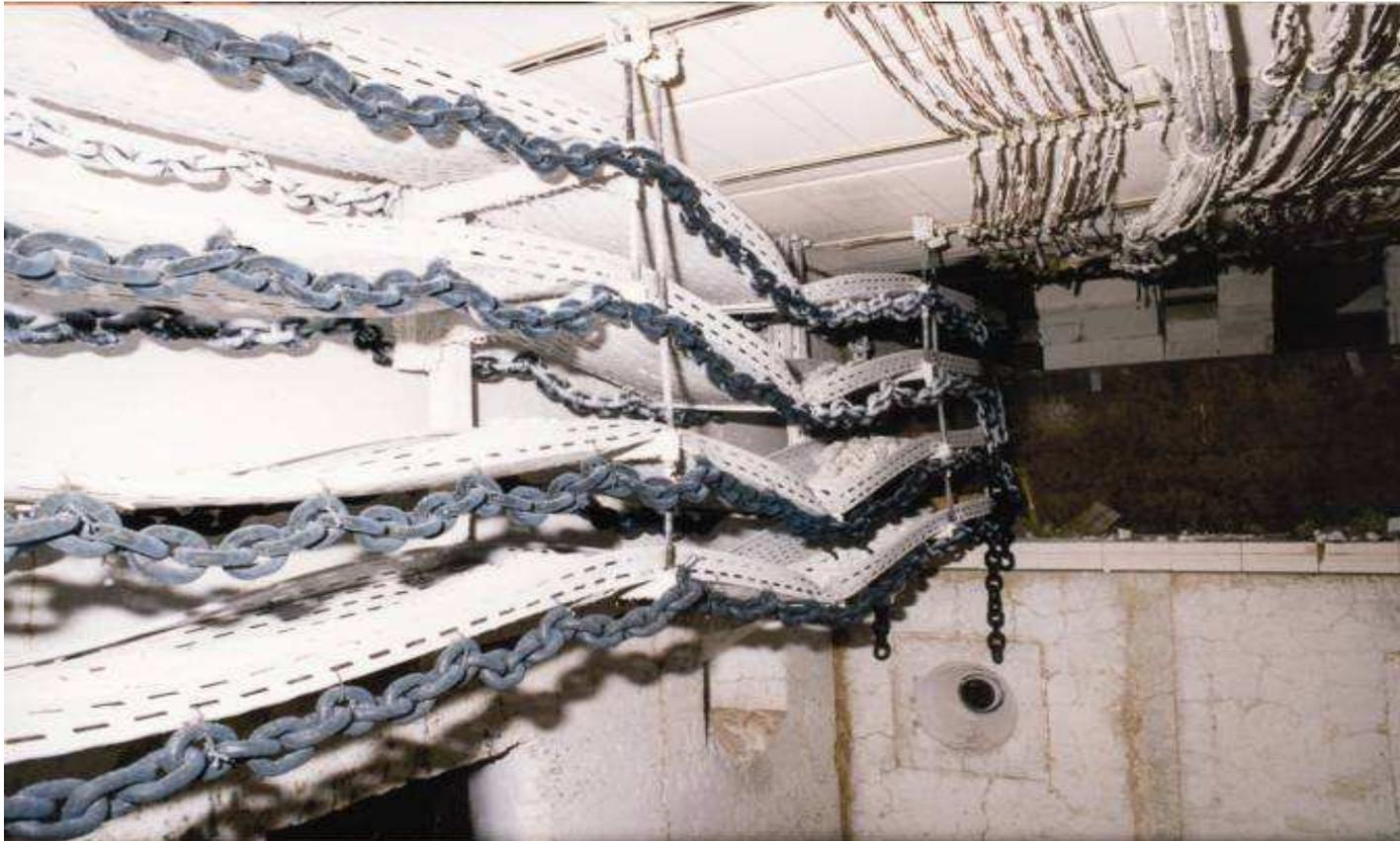
**E 90 Cable Weight 20 kg/m Support Span 1,5m**
